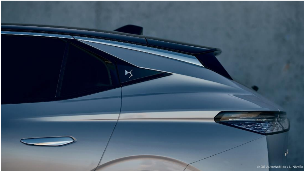
PLEXIGLAS®, the brand PMMA from Röhm, can be formed into almost any shape using injection molding: The lines of the DS 4 body continue into the three-dimensional taillights. © DS Automobiles / L. Nivalle
