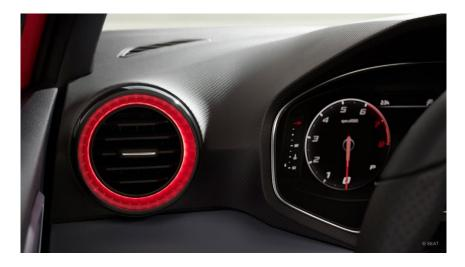
Air, light and color: SEAT has equipped the Ibiza and Arona models with colored, illuminated air vents. The components are made using the PLEXIGLAS® LED LD special molding compound from Röhm.
