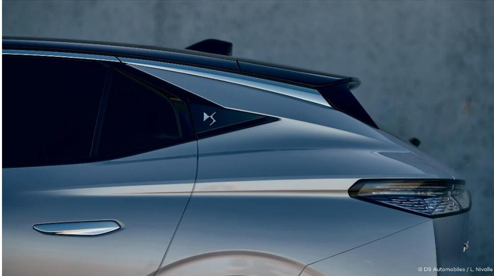
ACRYLITE®, the brand PMMA from Röhm in the Americas, can be formed into almost any shape using injection molding: The lines of the DS 4 body continue into the three-dimensional taillights.
