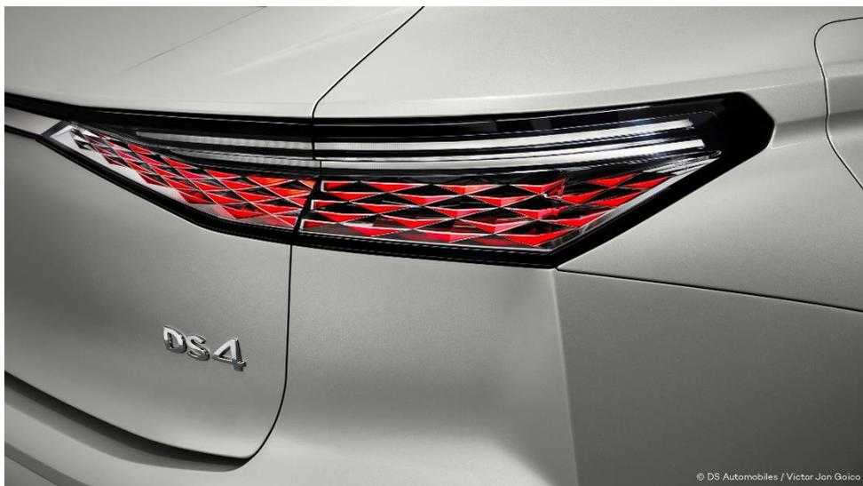
The taillights of the DS 4 are reminiscent of a jewel. The characteristic multifaceted design of the lenses is created using a metalizing process and laser etching. The shimmering cover made from ACRYLITE® molding compound completes the high-quality overall image, while the high-gloss contour made from ACRYLITE® Hi-Gloss 8N black ensures the taillight covers flow seamlessly into the car body.
